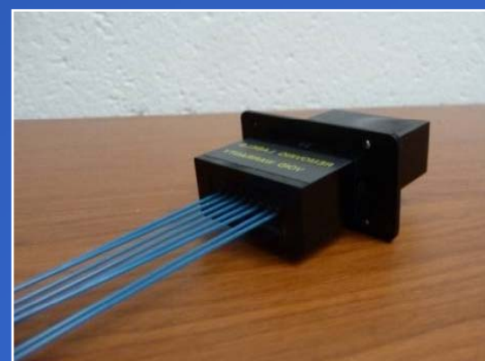
8-channel fiber coupled PMT
